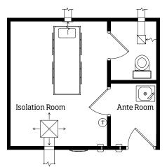
One PresSura display unit monitoring isolation room and ante room simultaneously.
